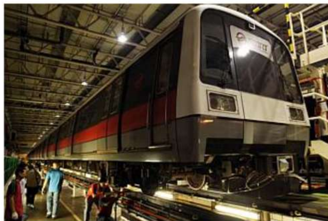
SMRT staff measuring the distance between the collector shoe and third rail on one of the trains at the Bishan Depot at 5.30am on Dec 18. SMRT only conducted a thorough fleet wide inspection of its trains after the second train disruption incident on Dec 17, the Committee of Inquiry heard on Wednesday. -- ST PHOTO: LAU FOOK KONG
